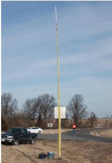
Portable digi with mast, battery, and pace vehicle with tracker passing by.
